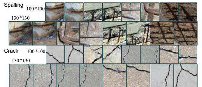
Fig. 4. Examples of generated positive training images based on proposed selection criteria. The spalling images are presented with size of  $100 \times 100$  with  $k = 0.04$ , and  $130 \times 130$  with  $k = 0.06$  for training. The crack images are also presented with  $100 \times 100$  with  $k = 0.04$ , and  $130 \times 130$  with  $k = 0.06$  for training.
