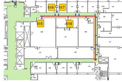
Figure 7. An arbitrary route is designed for the test. The blue segments indicate the landmarks to be passively detected along the path.
