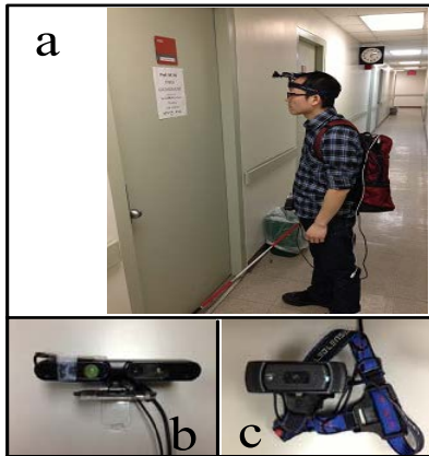
Figure 1. The proposed wearable system is composed by backpacked laptops, a microphone, a speaker, a RGB-D sensor with IMU and a head mounted camera.
