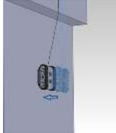
Figure 4. Duct fans push the robot in contact with wall surface.
