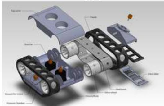
Figure 2. Exploded view of the Rise-Rover robot.
