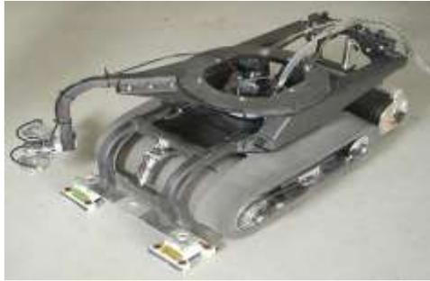
Figure 1. ICM robot uses rolling seal and AC suction pump for strong adhesion.
