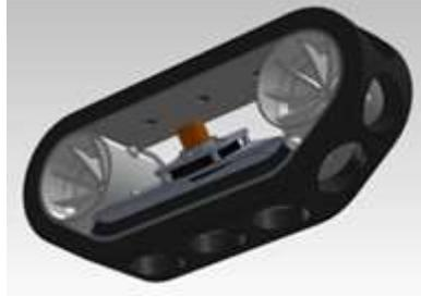
Figure 3. A drivetrain with foam tread and vacuum rotor package.
