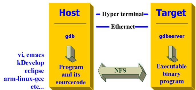
Fig. 6 Development environment of embedded linux
