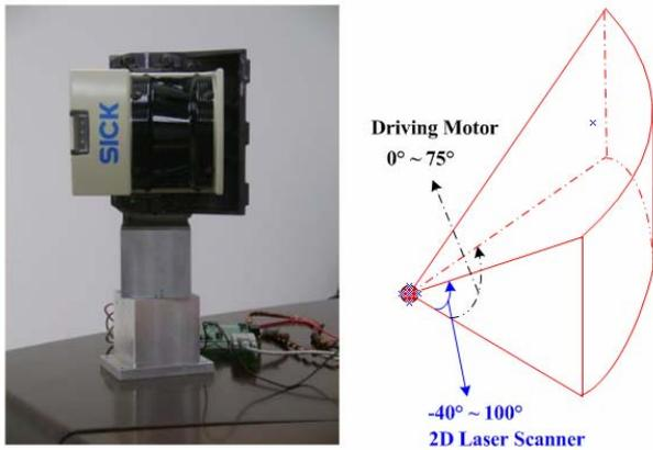
Fig.1 LMS291 laser scanner and motor driving motor
