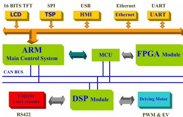
Fig.2 Structural diagram of embedded system
