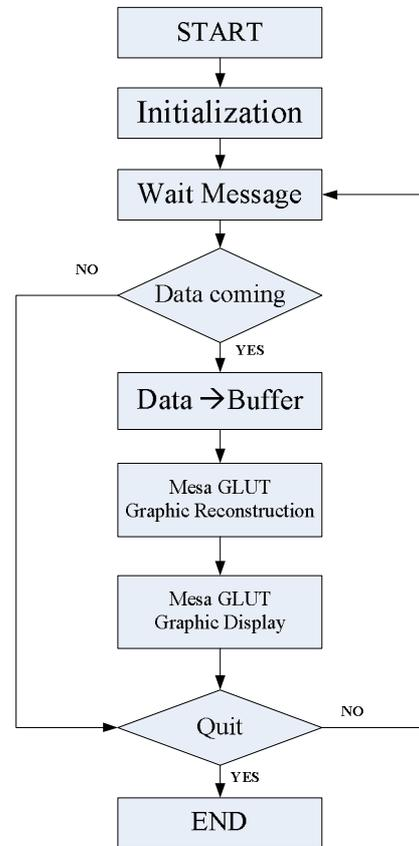
Fig. 7 Flow chart of 3D reconstruction
